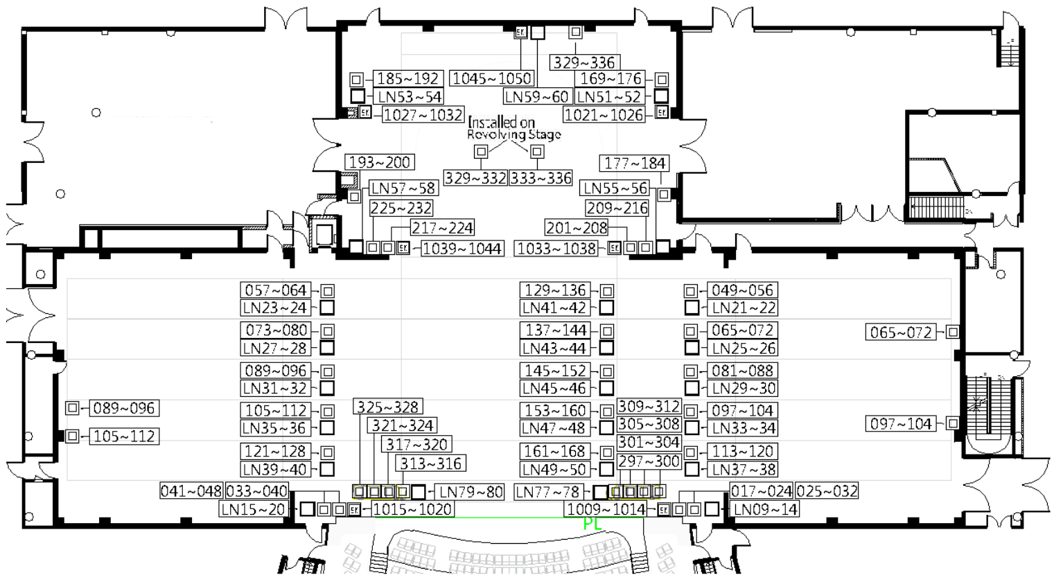
Figure 2.3.1.1- First Floor Lighting Circuit Layout
